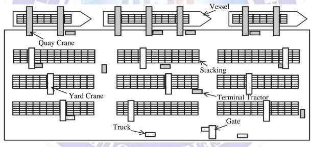
Figure 1: A container terminal and its equipment (Sun et al., 2011)
